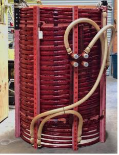
Induction furnace coil supports are made of unique glass fiber composites.
